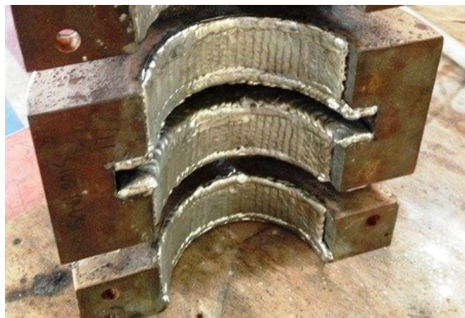
Bearing coated with Babbitt 90 SN using GTAW
