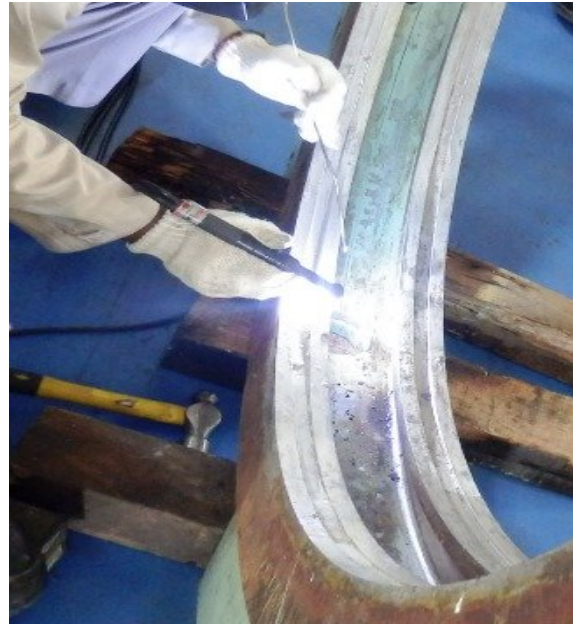
Welder applying Babbitt with GTAW Process
